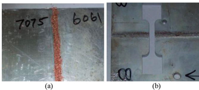
FIGURE 4.—(a) Copper particles packed in faying sides. (b) Root side of the weldment (color figure available online).
