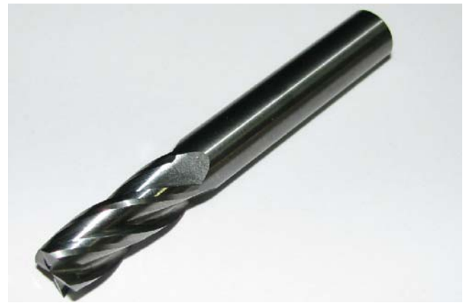
Fig. 18 Sample of an end mill machined using the developed software
