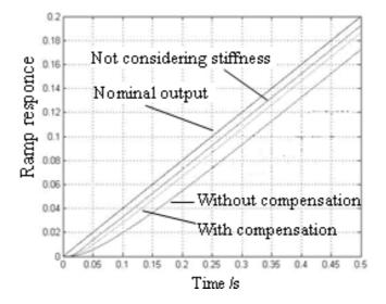
Fig. 7. Ramp response of the feed system.
