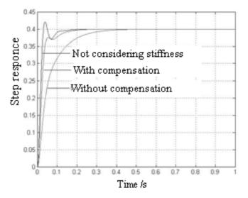
Fig. 6. Step response of the feed system.
