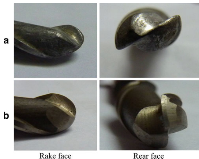
Fig. 10 The rake face and rear face a before and b after ground
