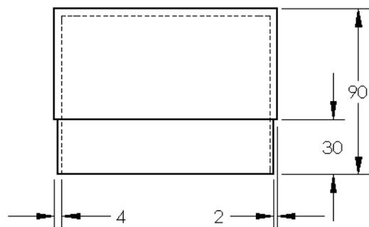
ESPESOR DE PARED = 4 mm
