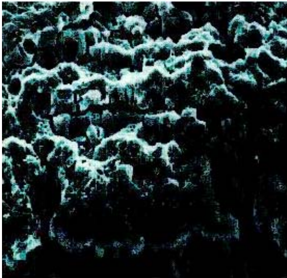
Figure 2-10. Grain Structure of a Corroding Aluminum Surface
