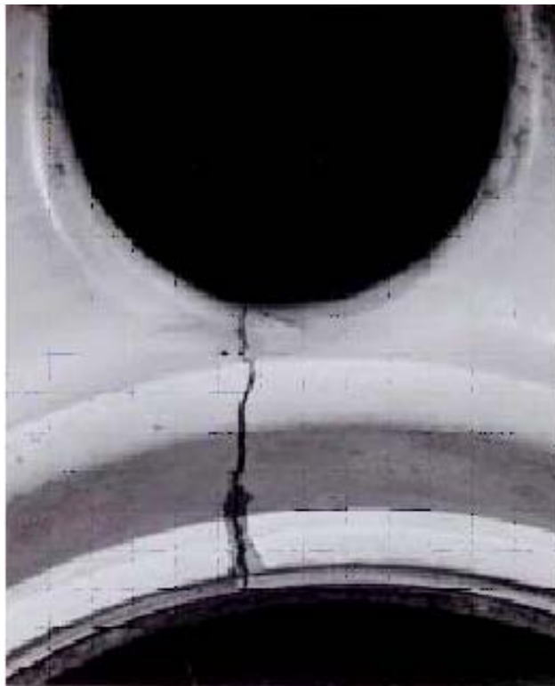
Figure 2-15. Stress Corrosion Cracking
